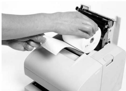
5. Pull out the leading edge of the roll paper; then close the roll paper cover until it is firmly locked by pushing the top of the cover.
