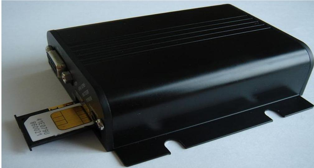
PS. If you want to replace the SIM card, press the push button and pull out the holder. Be sure the SIM card can support the GPRS service.
