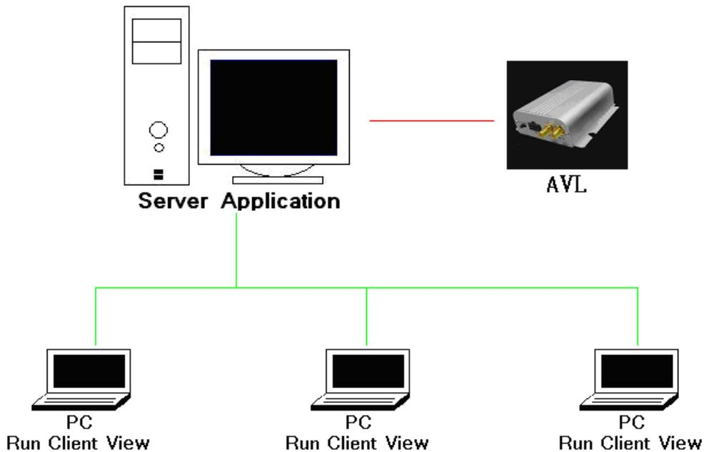
The AVL contains the GSM/GPRS module and will send the location information to the Server.
