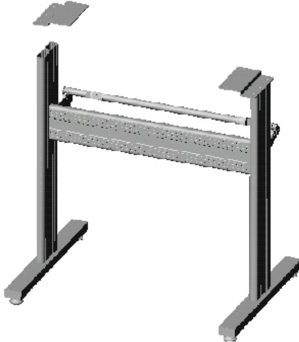
Step 1: Rotate the stand pillars into screw thread-holes in the pillar bars, and then connect the pillar bars to left and right columns with screws respectively.
