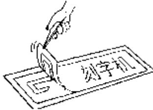
3. Adhere a special “over-pasted film” on the cut pattern and stroke it with a scraper.
