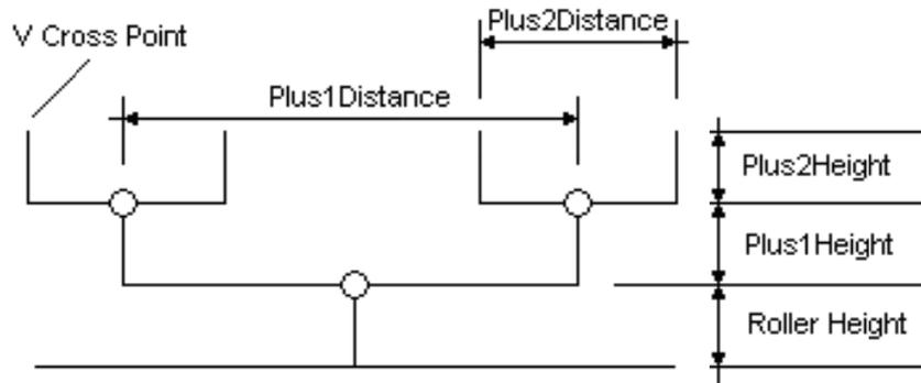
Fig. 3.8 Definition of roller height and plus height
