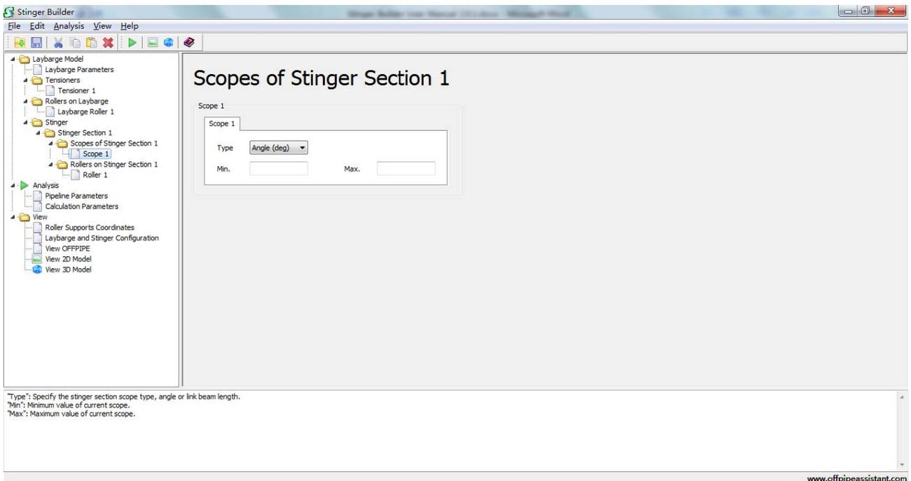
Fig. 3.15 Input parameters for each scope of the current stinger section
