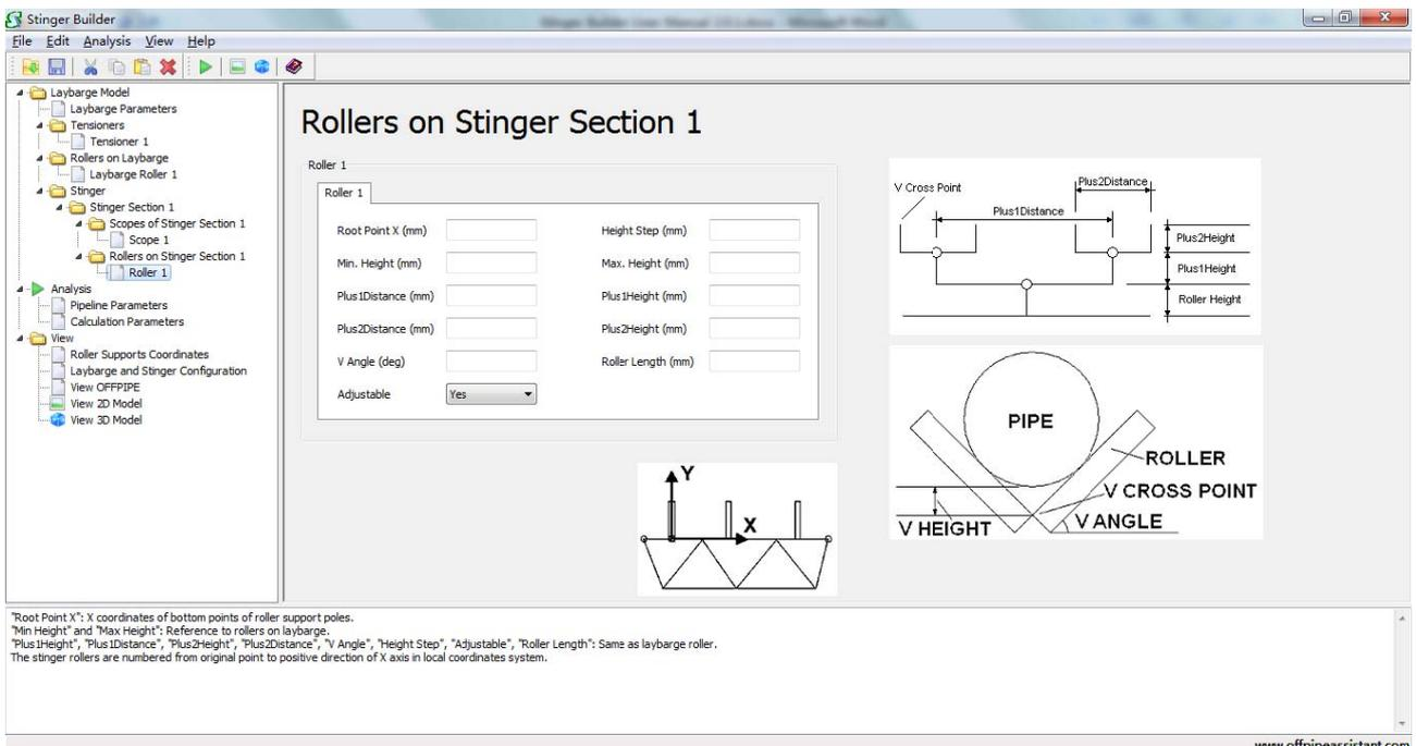
Fig. 3.17 Input parameters for each roller on the current stinger section
