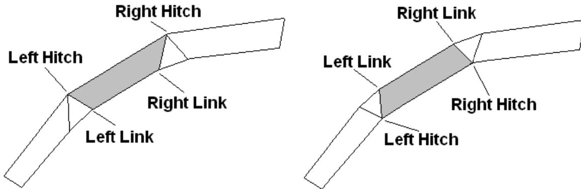
Fig. 3.12 Definition of hitch and link point
