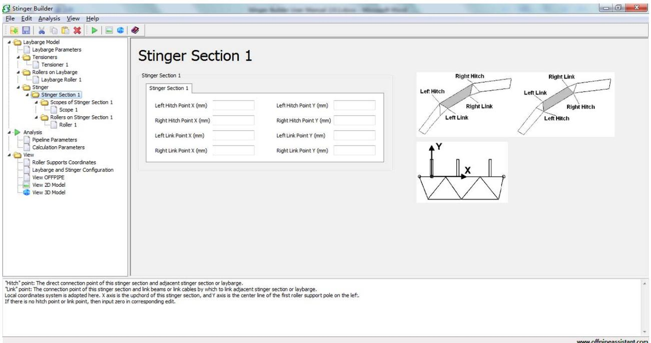
Fig. 3.11 Input parameters for each stinger section
