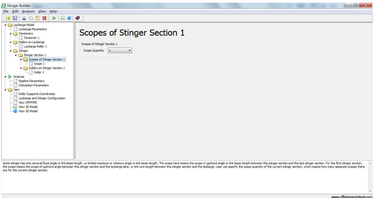
Fig. 3.14 Specify scope quantity of the current stinger section
