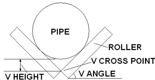
Fig. 3.9 Definition of V angle and V cross point
