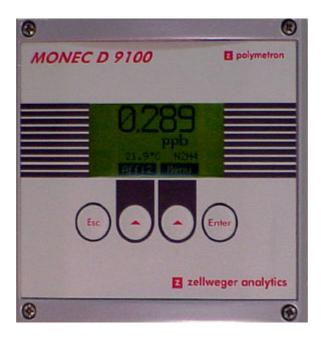
The electronic unit amplifies the signal of the amperometric measuring cell and converts it into a direct digital readout in ppm, mg/l, ppb,  $\mu$ g/l,  $^{\circ}$ C and  $^{\circ}$ F. The transmitter comprises the following items :
