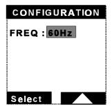
You can program the mains supply frequency at 50 or 60Hz.
