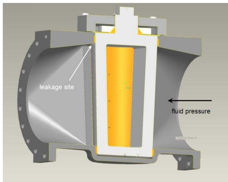
**Figure 2.1.** Leakage site upon testing of the valve.
