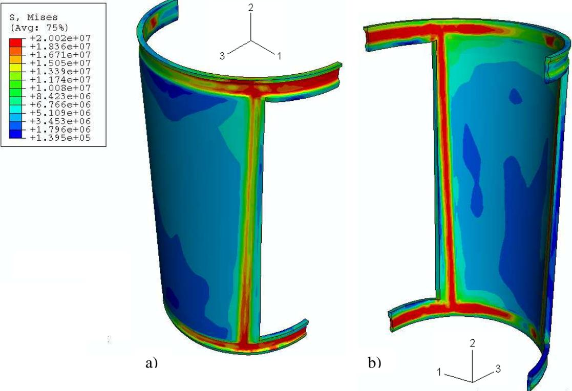
**Figure 5.5.** Von Mises stress distribution in the sleeve after the fluid pressure has been applied, before the stress relaxation has taken place, a) outer surface and b) inner surface.
