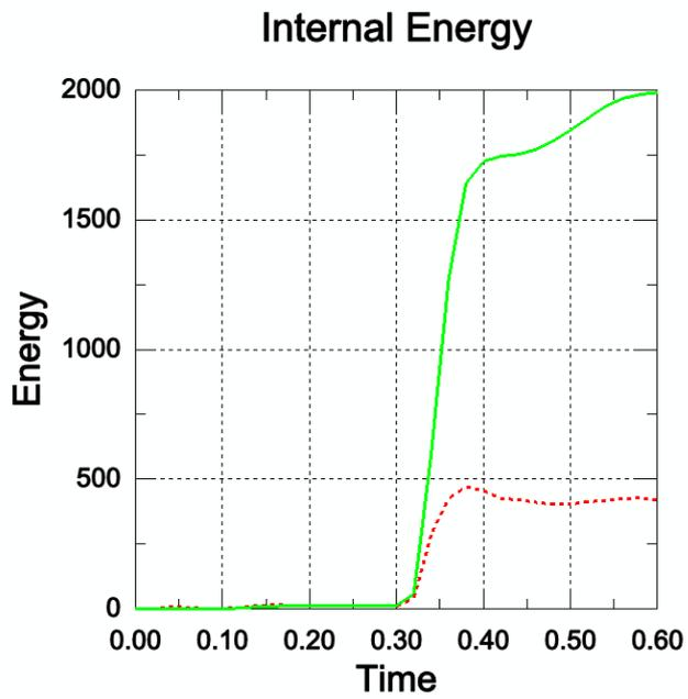
**Figure 5.3.** Internal energy during assembling and fluid pressure application.
