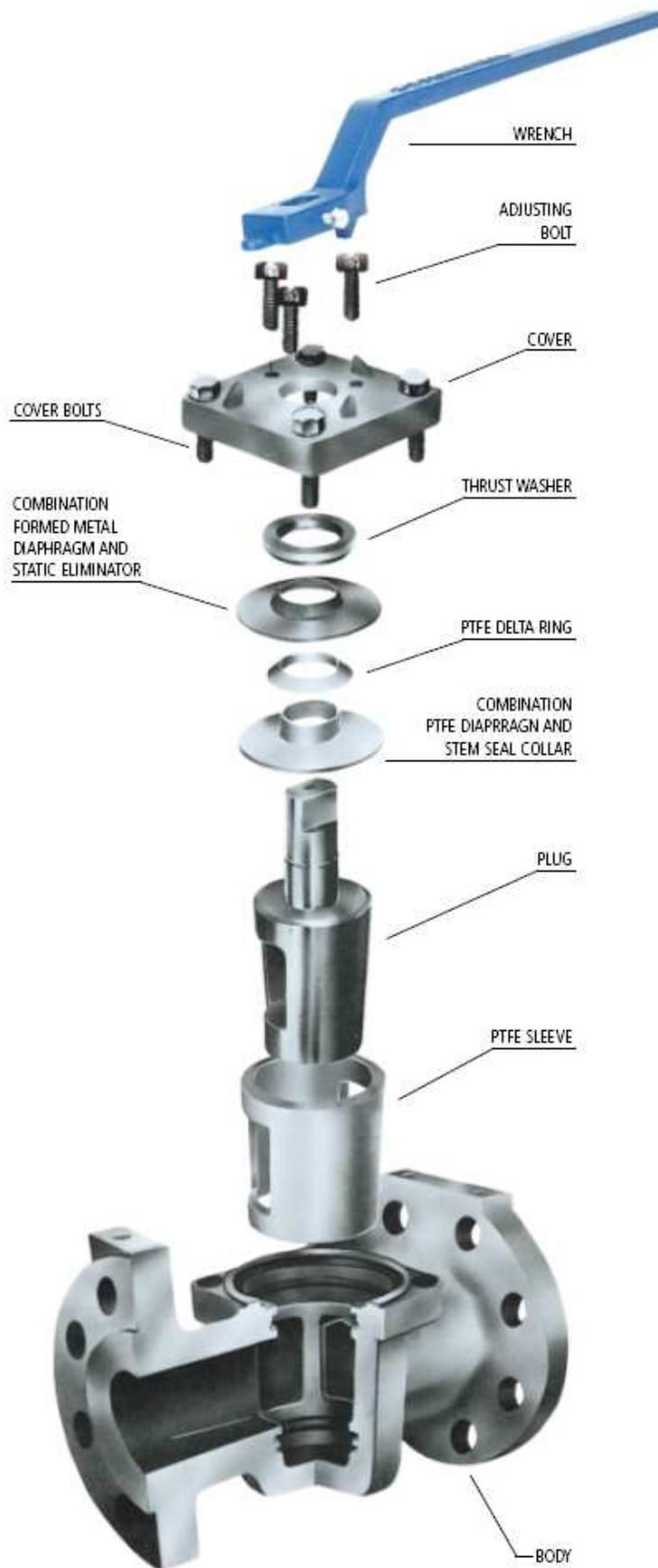
**Figure 1.1.** An explode view of a Fluoroseal plug valve.
