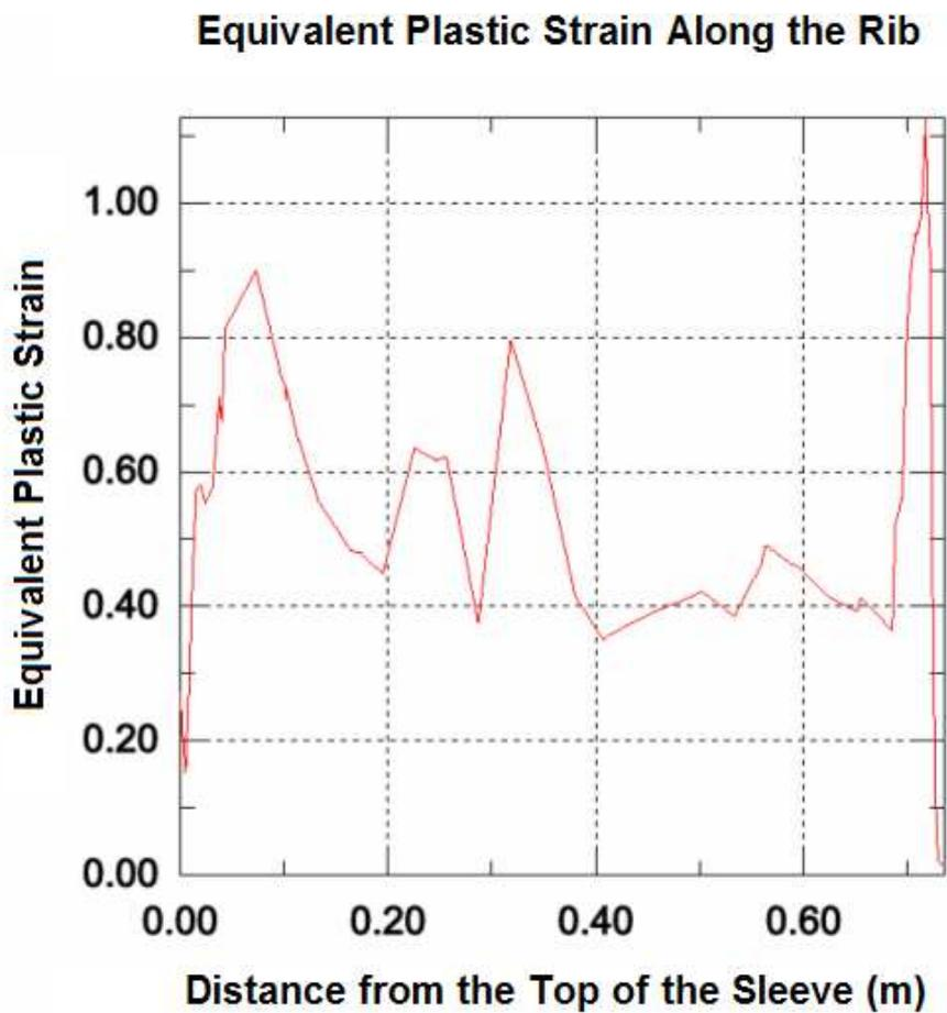
Figure 5.9. The equivalent plastic strain along the rib, where the leakage occurs.
