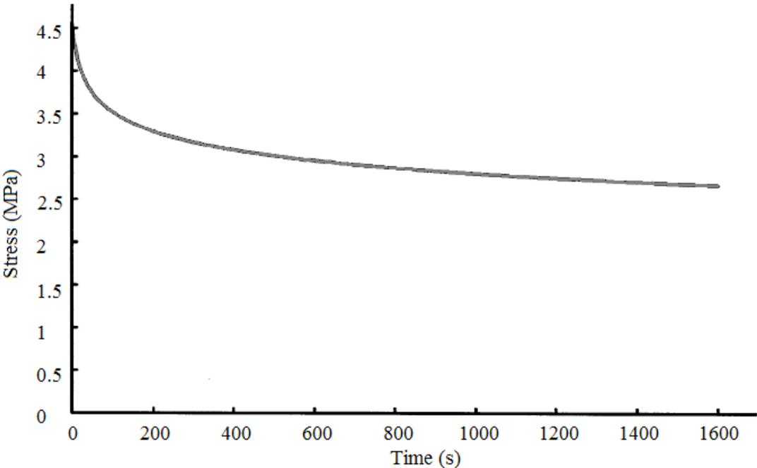
Figure 3.5. Stress relaxation behavior for a PTFE test specimen [2].
