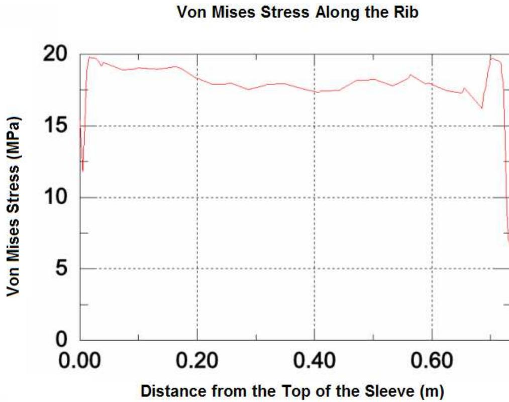
Figure 5.8. The von Mises stress along the rib, where the leakage occurs.
