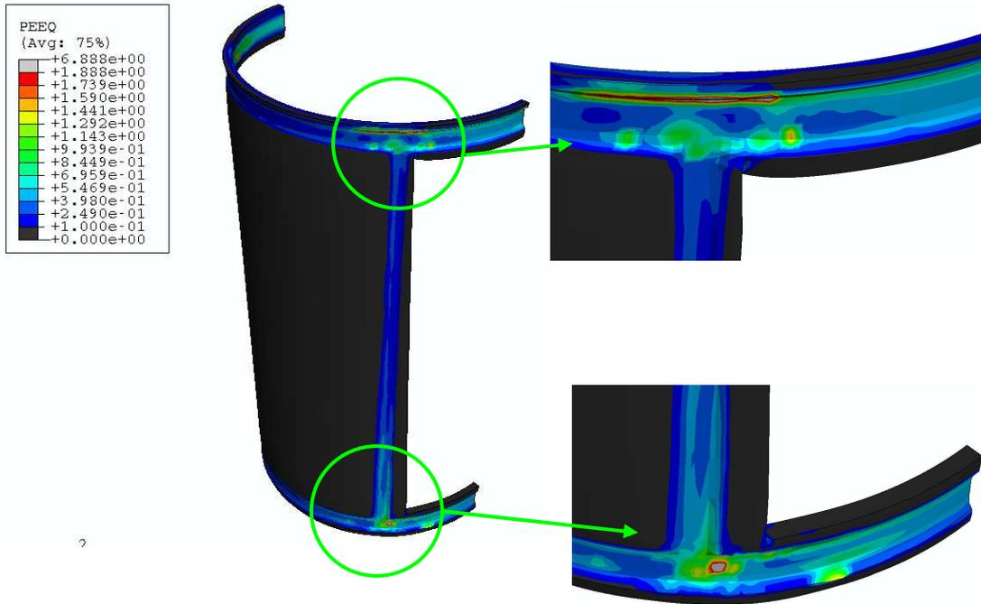
**Figure 5.6.** Plastic strains in the sleeve after the fluid pressure has been applied, before the stress relaxation has taken place.
