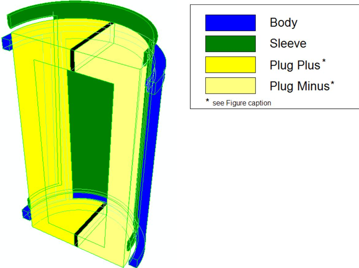
**Figure 4.2.** The geometry used in the finite element model. The plug is cut into two halves, labeled “Plus” and “Minus”, in order to facilitate the assemblage.
