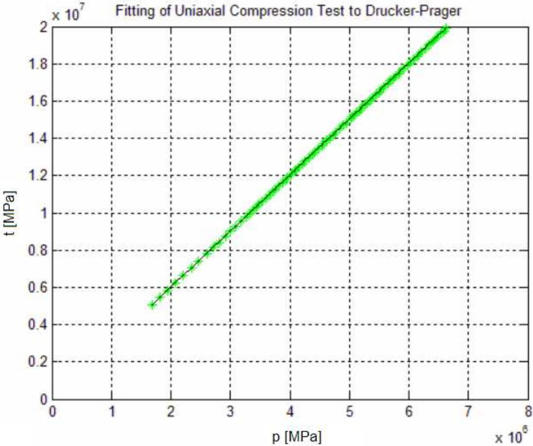
**Figure 4.4.** Curve fitting of test data to the Drucker-Prager constitutive model.
