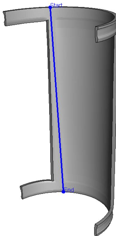
**Figure 5.7.** The path, corresponding to the rib, along which the stresses and strains are plotted.
