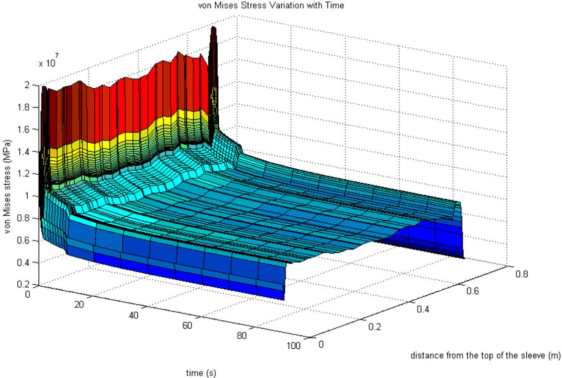
**Figure 5.10.** The von Mises stress variation during 90 seconds after the fluid pressure application.
