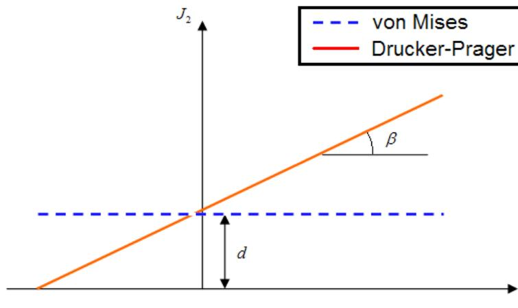
**Figure 3.4.** The meridian plane for the von Mises and the Drucker-Prager criterions.
