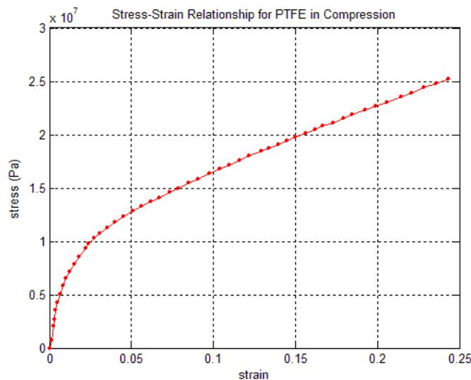
**Figure 3.3.** Stress-strain relationship for PTFE in compression at room temperature and a strain rate of  $10^{-4} \text{ s}^{-1}$ .
