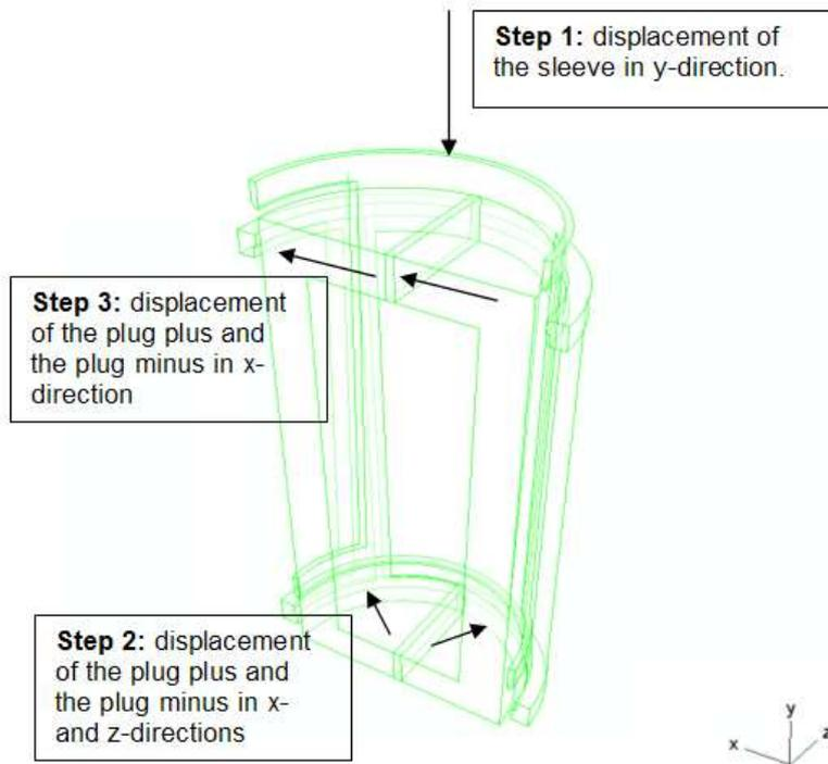
**Figure 4.5.** Displacements of the parts by assigning non-zero boundary conditions.
