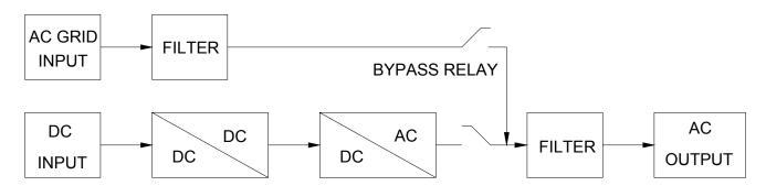
The inverter features IGBT technology which, minimizes weight and dimension, while enhancing output short circuit reliability and overload capacity.
