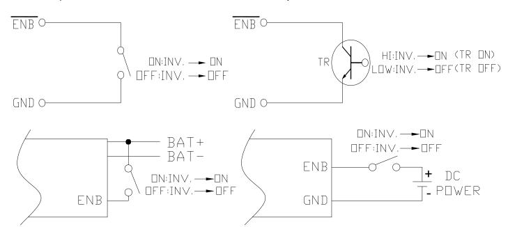
NOTE: At one time, only one remote function should used to control the inverter. The maximum voltage value is 60VDC.
