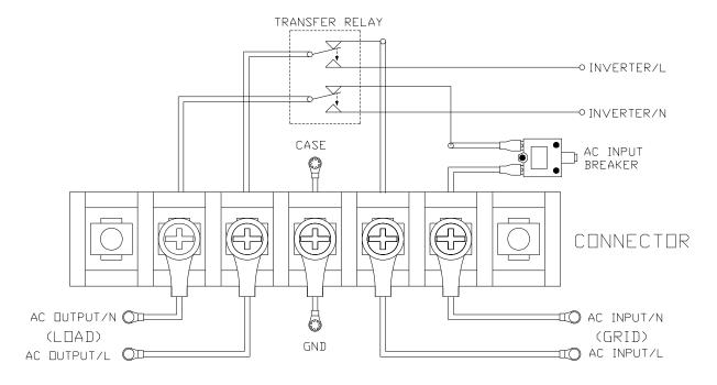
■ Connect AC output and AC input wiring to the Inverter terminals. Please use the following information as your reference:
