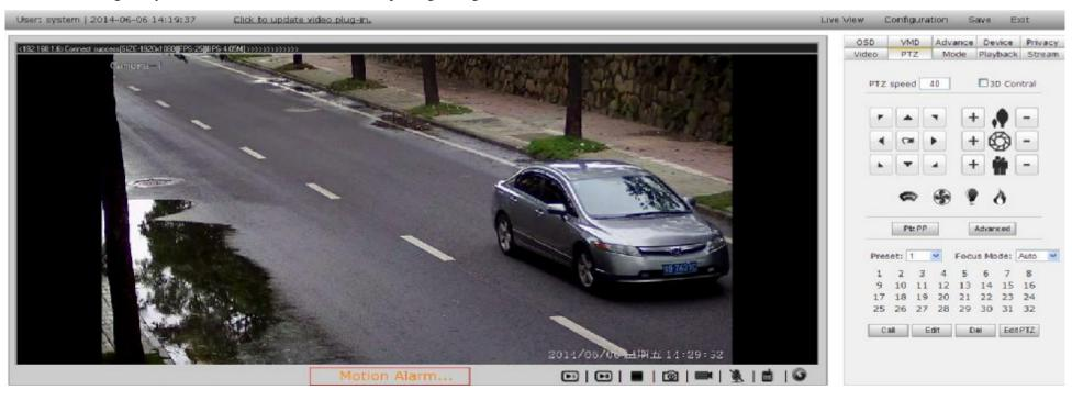
3.15.9 If you prefer MJPEG as second video stream, setting from "Live view - Stream - Stream Type - Second video stream setting- Setup - Save". Step 1-6
