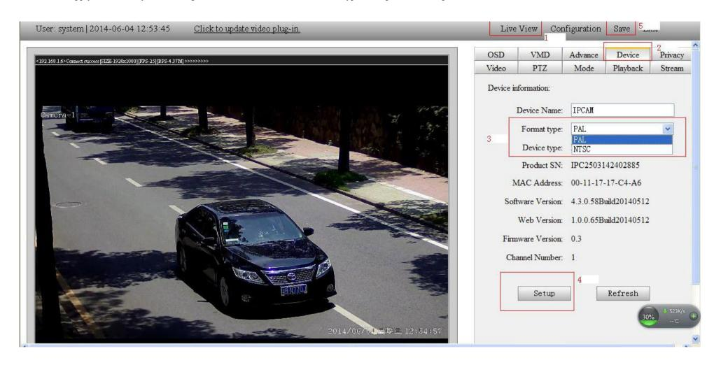
3.15.12 Manual recording, "Live View", Press recording icon to start and stop. Find recording at D:/Record/Video on your computer. It is for test purpose.
