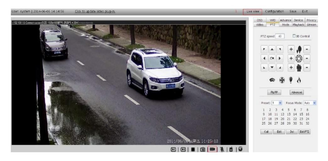
3.15.13 Manual snapshot images, "Live view" Press image icon to start capture. Find images at D:/Record/Image on your computer. It is for test purpose.
