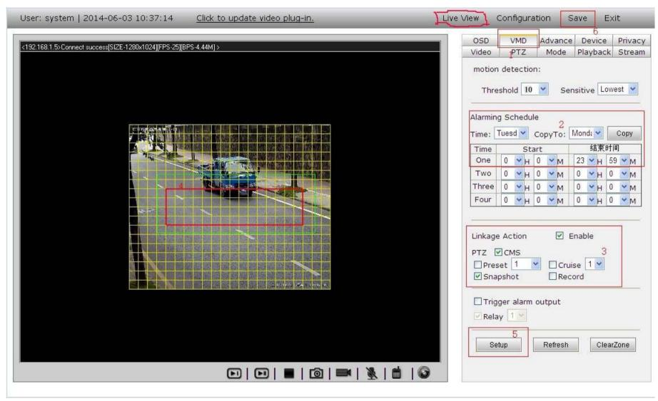
After finish VMD setting, it shows "Motion Alarm..." when the car is passing through the virtual square area.
