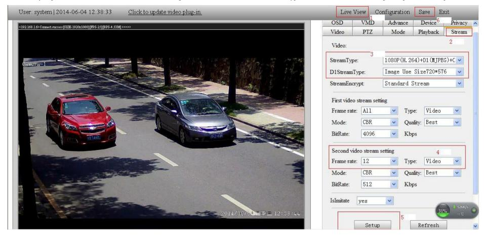
Remarks: When sub video stream is MJPEG, can't set higher frame rate of real time view. The camera can't proceed high stream. It will restore from time to time because of high stream.
