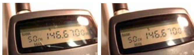
Scratch on plastic scanner dial indicated by arrow (left) was largely removed by rubbing with Krazy Kloth (right).
