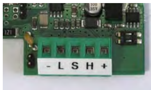
terminal and jumper for WDESK-P/X and WINOX-P/X instruments
