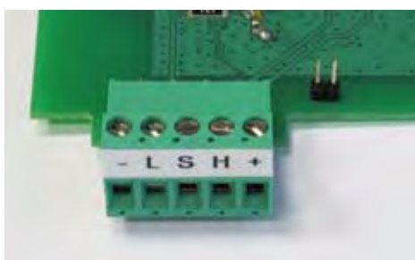
terminal and jumper for W200/W200BOX and WDOS instruments
