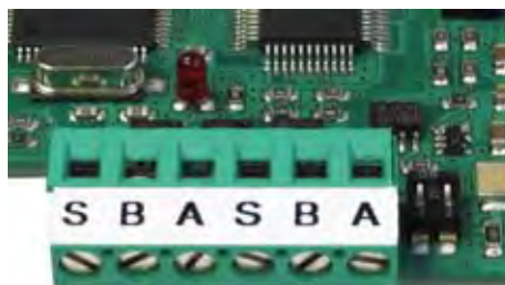
terminal and dipswitch for WDESK and WINOX instrument
