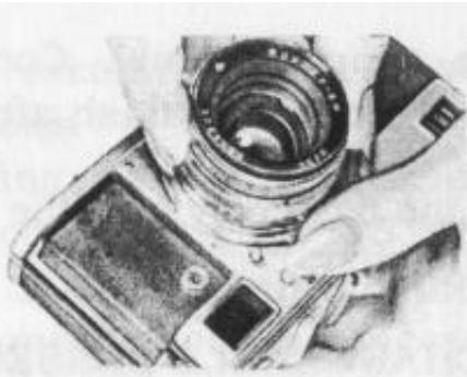
Fig. 19. Removing a lens F = 5 sm.
