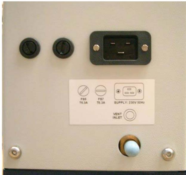
The 2 mains supply fuse holders F6 and F7 are standard screw type located next to the mains power connector on the left hand side of the evaporator (viewed from the front).
