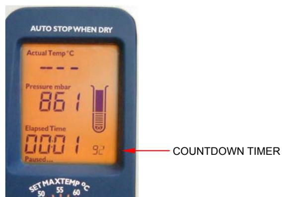
System will vent and stop the rotor, countdown timer will count from 96 down to 0. The lid can then be opened and the samples examined.
