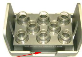
Locate sample blocks correctly in sample swings.
