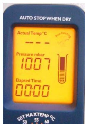
If the system enters pre-heat / pre-cool mode then the rotor will spin up.
