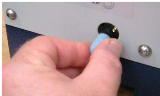
10. Fit CatchPot (Not on EZ-Bio – refer to separate sheet supplied with evaporator).
