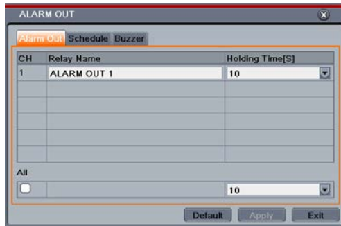
Fig 5-22 System Configuration-Alarm Out
