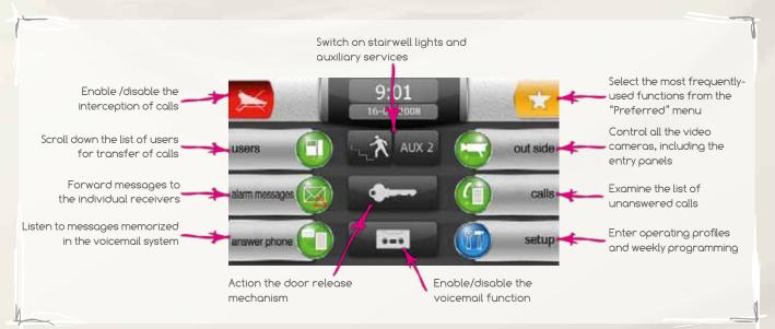
When a call is received from one of the entry panels, the switchboard operator is advised by a customizable ringtone melody and receives the video image from the entry panel. At this point, the operator may:
