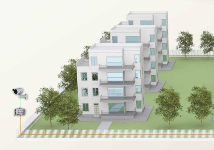
Systems for medium-sized residential complexes can be created using the backbone connecting the main entrance point(s) and the individual residential units (houses and/or blocks), using a normal non-polarized twisted pair (or, for maximum performance, it is possible to use Bpt's VCM/1D dedicated cable).
