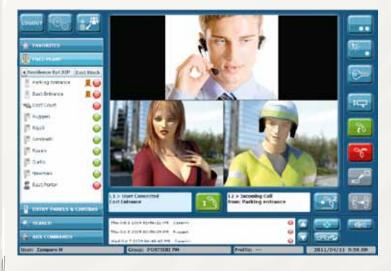
If a second call is received while another call is in progress, the images will be displayed as shown opposite. One of the two calls can be placed on hold at the touch of a fingertip.
