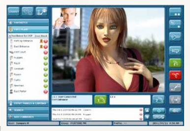
When a call is received, the image from the entry panel is displayed in full-screen mode on the porter's monitor; the image of the porter is shown in PIP (picture-in-picture) mode.
