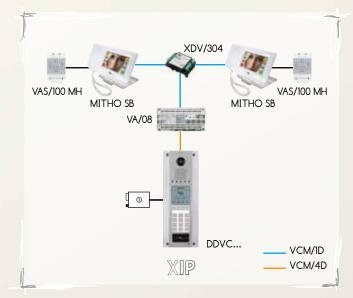
Mitho SB is a sophisticated solution for providing porter services in XIP systems in which LAN networks are not used.
