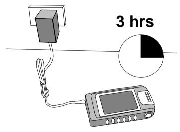
The red light beside the power connector should illuminate indicating that the battery is being charged. The light will go off when the battery is substantially charged. It takes about three hours to charge the battery from a discharged state. Quicklook Focus can be used while the battery is being charged.
