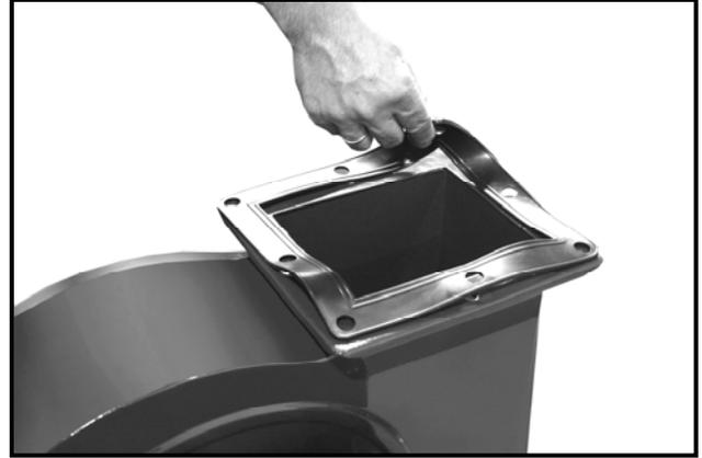
Figure-5 Placing the gasket on the motor flange
