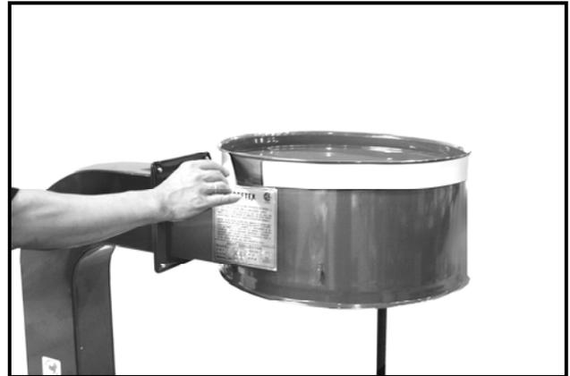
Figure-9 Attaching the foam strip to the top part of the collector
