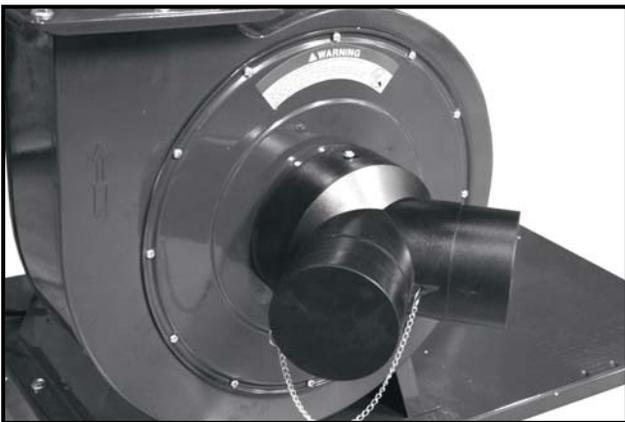
Figure-12 Installing the inlet connector
