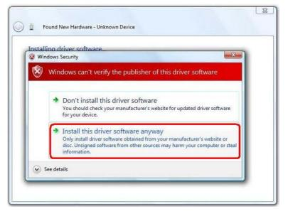
6. During installation of the driver software it shows a security issue that Windows can't verify the publisher of this driver software. Click at the option "Install this driver software anyway"
