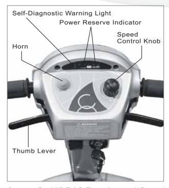
Figure 2 - HS-360 Top Control Panel
