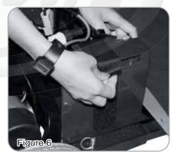
Detach Battery Power Plugs.(See Fig. 7) Remove two Batteries.(See Fig. 8)
