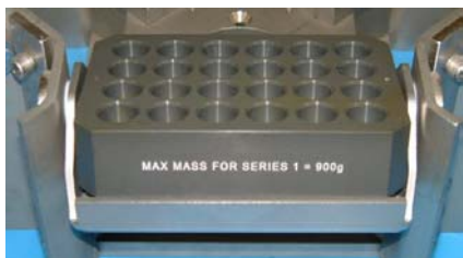
Incorrect – Sample Holder on edge of swing
