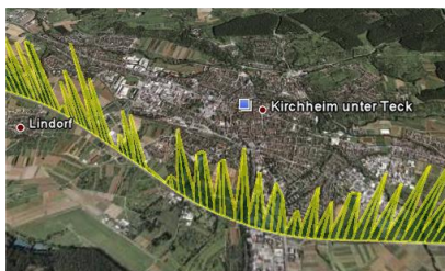
Figure 15: Data throughput rates created with the use of CAR-A-WAN.automotive / .coach and Google Earth.
