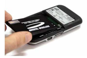
Gonnect the wall charger to MiFi and charge for a minimum of 4 hours before use. The power button LED will flash amber while the device is charging and glow solid amber once charging is complete.
