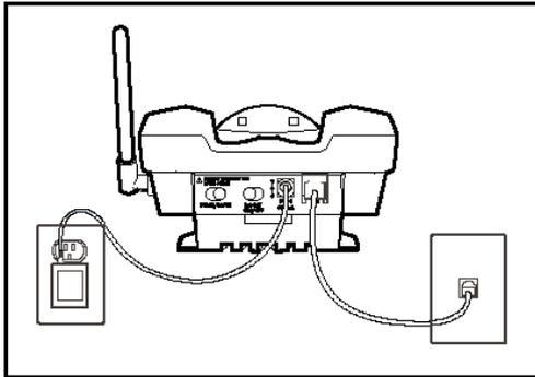
The power adapter and telephone line ports are located on the back of the base.
