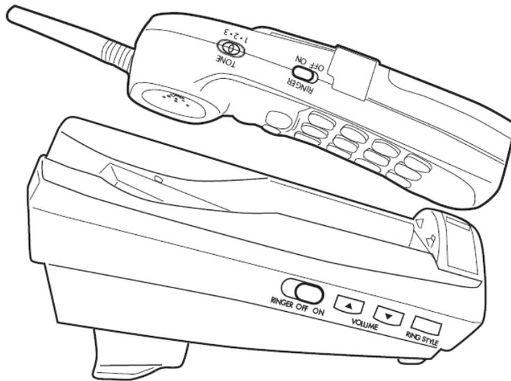
Install battery by removing battery door on back of handset and connecting the white plug into handset.
