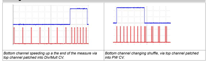
This is an easy patch with the QCD. Just run the INV OUT of a slow channel (/8, for example) into the Div/Mult CV jack of a faster channel (x4, for example). Set the slower channel's Mode Switch to center (Inverted Gate mode). Turn the faster channel's Div/Mult CV attenuator slightly to the right of center to set how fast the fill will be. Adjust the slower channel's Gate PW to set the length of the fill (number of beats).
