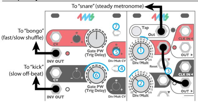
This patch uses the black channel to speed up and slow down the red channel. The black Div/Mult (2) determines how quickly the red channel changes from fast to slow and back. The black PW (5) determines how long it's fast vs. how long it's slow. The red Div/Mult (11) determines the slow speed, and the CV attenuverter (4) determines the fast speed. After patching, we should hear bongos speeding up and slowing down and a kick whenever the bongos change tempo.
