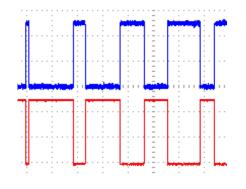
Inverted Gate Mode: Top trace (blue) is main QCD OUT. Bottom trace (red) is INV OUT. PW/Trig Delay being swept from 0% to about 75%.
