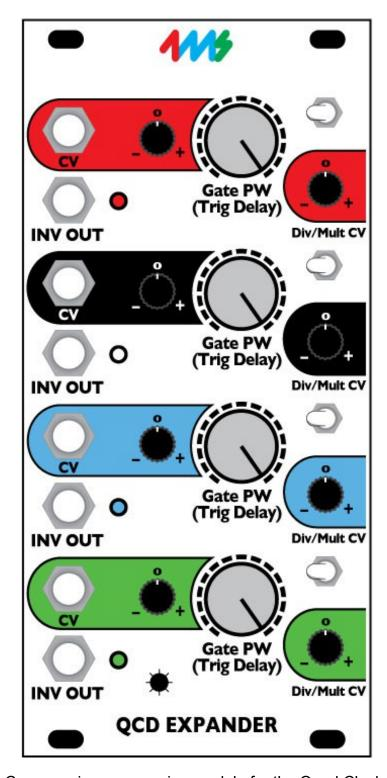
The QCD Expander from 4ms Company is an expansion module for the Quad Clock Distributor (QCD). The QCD Expander requires the QCD to function, and adds a host of features. The Expander turns the QCD into a programmatic non-linear sequencer, easily obtaining self-patched evolving rhythms, and swing/shuffle patterns.
