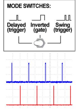
Delayed Trigger Mode: Top trace (blue) is master clock (shown as a trigger for emphasis). Bottom trace (red) is Delayed Trigger. PW/Trig Delay is at 50%.
