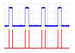
Inverted Gate Mode: Top trace (blue) is main QCD OUT. Bottom trace (red) is Delayed Trigger. PW/Trig Delay is set to 25%.
