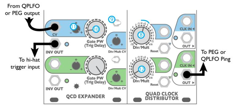
Now let's add some phase-shifting hi-hats. The blue channel is set to shuffle mode, and Trig Delay is modulated by a slow LFO or envelope, making the shuffle amount change over time. The green channel is set to a slow rate and should reset, ping, or trigger the external LFO/envelope.
