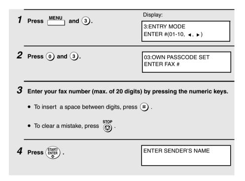
Flip the Rapid Key overlay down (if it is up), and enter your name by pressing the appropriate letter keys as shown below. (Max. of 24 characters.)
