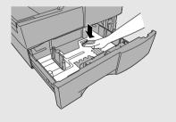
3 Squeeze the paper guide and pull up to move it to the appropriate holes for the length of the paper. Push the guide down into the holes.
