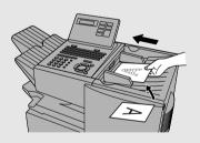
Note: When inserting a large number of pages in the feeder, slant the front end of the stack so that the bottom pages enter first.
