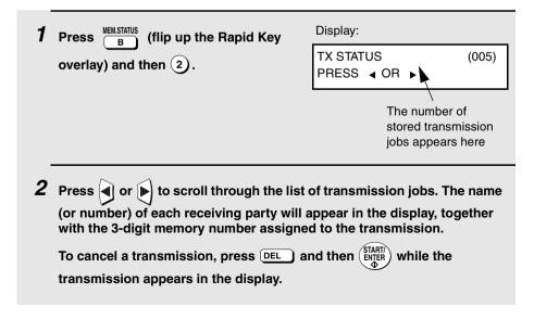
When you have finished checking the list, press twice to return to the date and time display.
