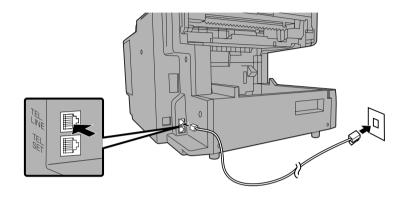
**Note:** The fax machine is set for touch-tone dialing. If you are on a pulse dial (rotary) line, you must set the fax machine for pulse dialing by changing Option Setting 22. See page 107.
