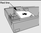
3 Squeeze the paper guide and move it to match the length of the paper you are loading.
