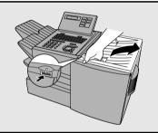
2 If you are replacing the toner cartridge, remove the old cartridge and dispose of it according to local regulations.
