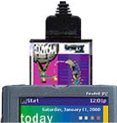
Plug the WWC directly into a CompactFlash I/O card slot
