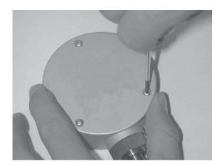
When in continuous operation (without light), the service life of the batteries is 1,500 hours. A battery symbol permanently displays the actual battery status.
