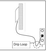
coming in contact with the receptacle. If the plug or the receptacle do get wet DO NOT unplug the cord. Disconnect the fuse to the circuit breaker that supplies power to the appliance. Then unplug and examine for the presence of water in the receptacle.
