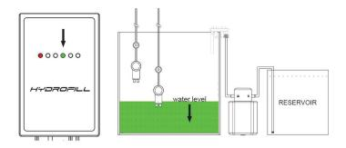
2. Only one sensor detecting water, controller shows LOW, pump is turned OFF
