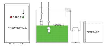
1. Both sensors detecting water, controller shows LEVEL, pump is turned OFF
