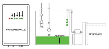
3. Both sensors NOT detecting water, controller shows 5 PULSING LEDs, pump is turned ON
