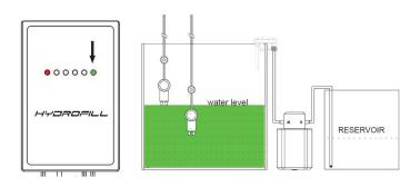
5. Both sensors detecting water, controller shows LEVEL, pump is turned OFF
