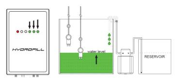
4. Only one sensor is detecting water while filling, controller shows 3 PULSING LEDs, pump is turned ON
