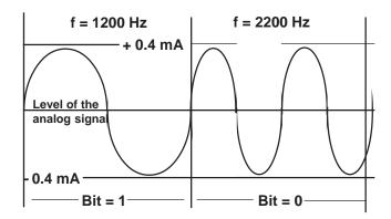
Since the energy balance added to the current loop is virtually equal to zero and the frequency used for the communication is very high compared to that of the process dynamic, no disturbance or interference occurs on the analog process signal.
