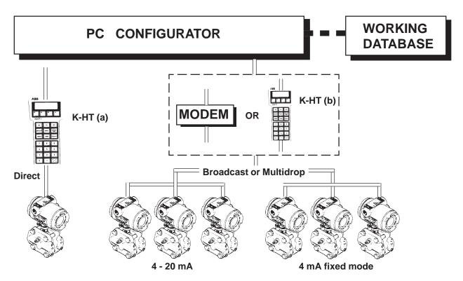
K-HT (a) is used to "transfer" configuration to/from field
