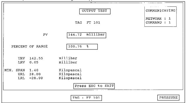
The **Tag**, the **PV** (Process Value) and the **Percent of Range** are displayed and **continuously updated** as shown by the Communication Box in the right top corner of the screen. If the transmitter's output exceeds its limits ( < 3.875 or > 21 mA) then the warning message "**Analog output saturated**" will be displayed. As usual use ESC to leave this option.
