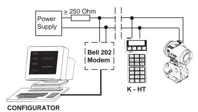
NOTE - A resistor of 250 ohm minimum must be present in the loop, between the HART connection and the power supply for communication purposes.
