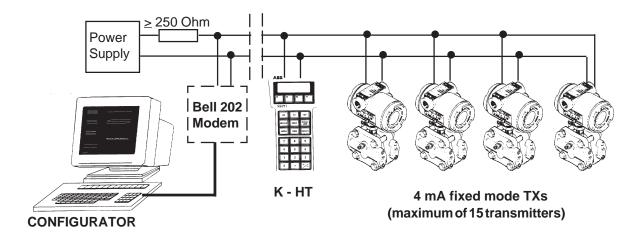
The connection should be done in parallel to the multidrop connected transmitter and is polarity independent. Also in this case, a resistor of 250 ohm minimum must be present in the loop, between the K-HT or the Modem and the power supply for communication purpose. The power supply should provide a minimum voltage of 12 Volt at the transmitters terminals and supply a current of 4 mA for each connected transmitter. A maximum of 15 transmitters can be connected in multidrop mode.
