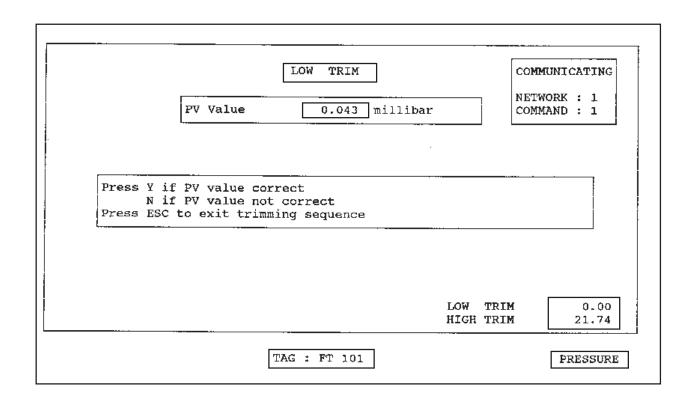
In the top right corner the screen presents the **Communication Box**, in the center, the **continuously updated PV** is displayed and in the lower right corner the values of **LOW TRIM** and **HIGH TRIM settings**. These values will be updated each time a trimming operation takes place. In case that the analog output is saturated the relevant message is shown.
