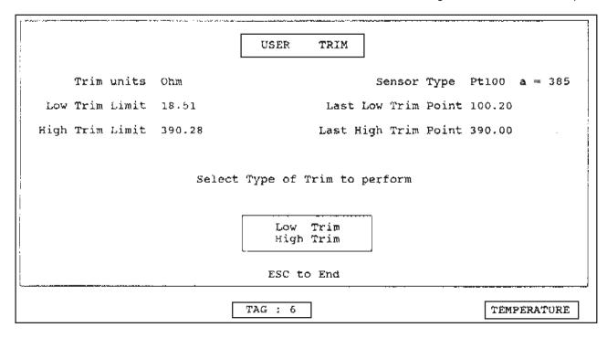
The procedures to perform a Low or a High Trim are identical: the following description covers the Low Trim operation. After making the selection the screen changes to User Low Trim and a box appears on the screen for some seconds with the message:
