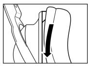
Turn the padding as illustrated. It will slide into the guide slot by itself. Keep turning it until it is correctly in place. Once it has taken on an oval shape, then it is correctly positioned.
