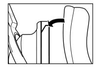
Bring the cloth padding up over the sloped guide slot. Hold it in place with your thumb just after the slope to ensure that it does not leave the guide.
