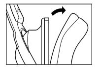
Carefully remove the cloth padding around the left and right headphones. Install the new batteries in their housings as illustrated. Check for correct +/polarity.
