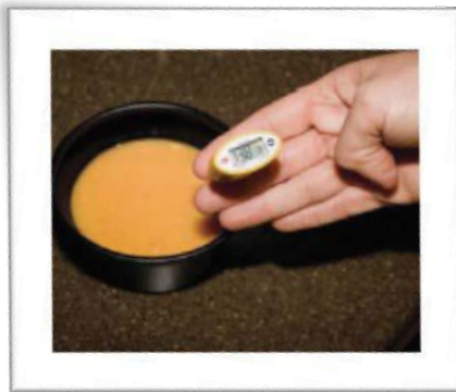
Bimetallic Thermometer (sensory area is from dimple on stem to tip)
