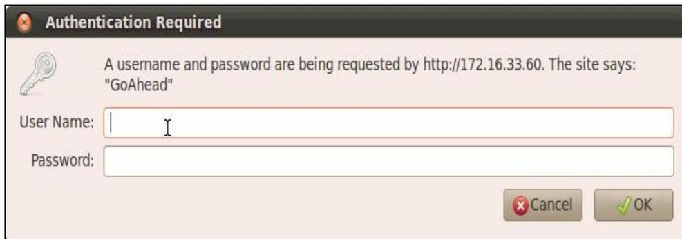
The default user name and password is "admin". To guarantee the system safety, when login for the first time. The system will prompt the user to modify the password. The interface is shown as below.
