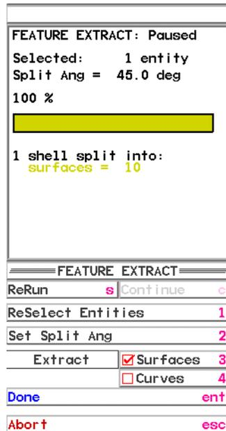
The Display window should look like Figure 25.3. The thick yellow lines in the Display window indicate the boundaries of the new shell surfaces resulting from the splitting operation.
