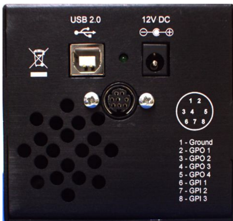
Figure 4 - Large Format Camera External Header Location and Pin Numbering
