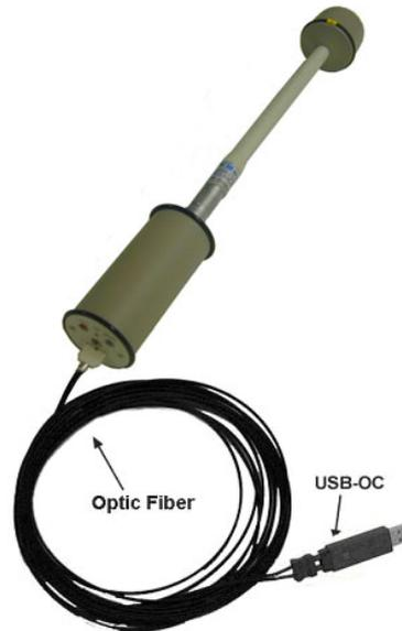
Fig. 4-1 OR03 link with USB-OC
