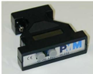
8053-OC is an optional accessory of the PMM OR03 Optical Programmable Repeater.
