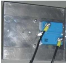
The resistors are mounted to the heat sinks to provide extra heat dissipation capacity. Each heat sink is large enough for two resistors.
