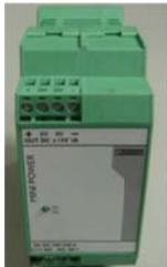
This supply takes a 120V AC input and creates a positive and negative 15V DC supply for the Hall effect sensors on the DC bus.
