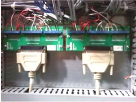
The boards provide termination points for the connections between the cDAQ and the Summit® DC power supply user cables. The 37 conductor cables are shielded to reduce noise, and the terminals on the breakout boards also allow sections of shielded cable to be installed to the final connections on the cDAQ terminals or the control relays.
