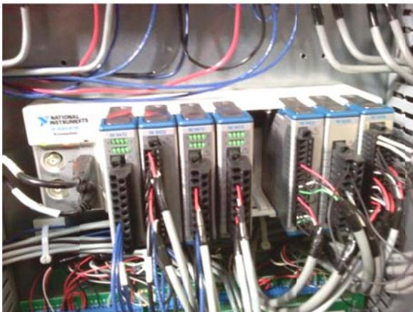
The cDAQ chassis communicates with the control PC through a USB connection, and runs LabVIEW programs executed on the PC. The cDAQ controls the DC power supply by sending signals through the user cables attached to the breakout boards located below the cDAQ.
