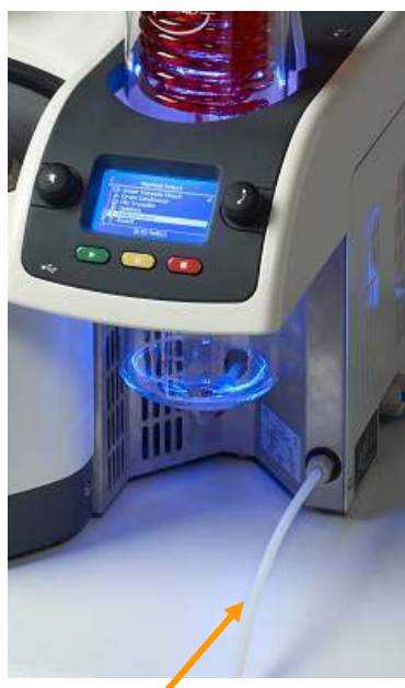
Waste solvent drain hose
