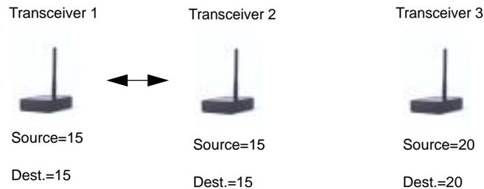
In a Multi-Point Network the Source for the Host PC is always zero and destination corresponds to the transceiver it is trying to communicate with in each session. It is a dynamic number. The remote units have the matching destination of zero but source numbers are unique.
