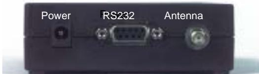
2. Insert Power supply plug into power (i.e., power outlet)
