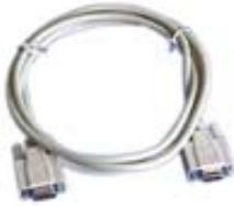
In order to configure any transceiver, you must use a 9 pin RS232 cable. This is necessary because pin 4 is used to transmit the configuration data into EEPROM and other pins are used during the configuration process as well. AirStream provides a 9 pin RS232 cable with all Stand-alone Transceivers. A TTL to RS232 pin adapter is purchasable for Design-in Transceivers.
