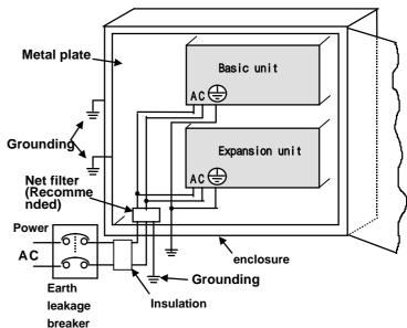
Figure 1 Power wiring example
