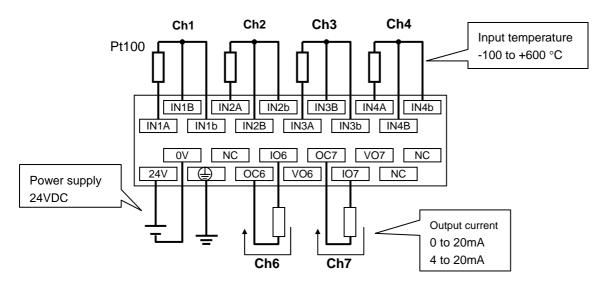
EH-A4ERTD (AC power, no analog output version) EH-D4ERTD (DC power, no analog output version)
