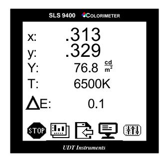
In the CIE 1931  $\Delta x \Delta y$  and CIE 1976  $\Delta u' \Delta v'$  modes, the reference is selected via the **DELTA REFERENCE** menu option in the **CONFIGURATION 2** menu (the bottom right icon, see page 3-13). Upon entry into this mode, the displayed delta values are calculated as follows:
