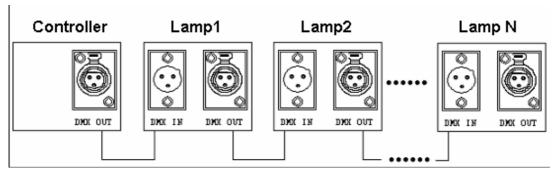
The shield connection is pin 1, while pin 2 is Data Negative (S-) and pin 3 is Data positive (S+).
