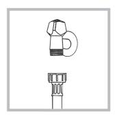
1. Connect the supply pipe by screwing it to a cold water tab using a ¾ gas threaded connection (see figure). Before performing the connection, allow the water to run freely until it is perfectly clear.
