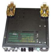
See a 6K16V viewed from the rear, at right, with model DIN-RAIL-VRM in place on the unit.
