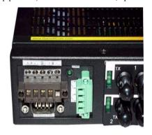
The second (bottom position) NC Alarm Contact is held close when there is power on the main board inside of the 6K16. This provides a "Hardware Alarm" because
