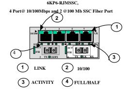
module of the 6K16-Series Switch supporting four Copper and two single-mode fiber network segments.
