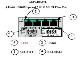
port supports fiber optic cable distances up the IEEE-standard 100Mbps distance limits, i.e., typically 2km at full-duplex and 412m at half-duplex.
