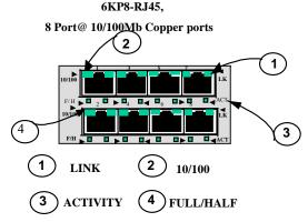
(MDI-X) switch, which controls all ports for cascaded connection. This feature eliminates the need for a special twisted pair crossover cable when connecting to a hub or another switch.
