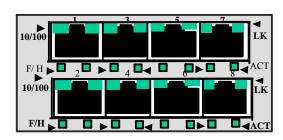
connected into an RJ-45 port and the Link (LK) indicator for that port must be ON (indicating there is a powered-up device at the other end of the cable) in order for a LK LED to provide valid indications of operating conditions on that port.
