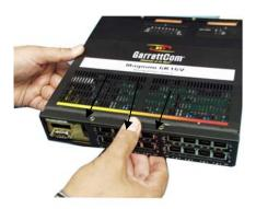
Figure 3.6.1a: Removing the Front panel from the unit
