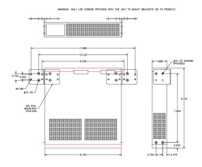
The unit can be mounted using the brackets turned outside (normal) or inside (if space is tight). Attach the mounting bracket either outside or inside as shown in the illustration above (dotted line shown for the brackets inside). The spacing for the mounting screws into the supporting wall or panel is a rectangle 11.89" x 7.85" center-to-center.
