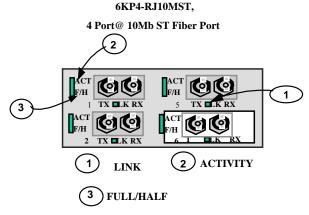
hub to connect to the switch through 10Mb fiber ports. It supports distances according to the 10Base-FL standard i.e, 2Km distance for multi-mode fiber. (Single-mode for 10Km distance may be available as
