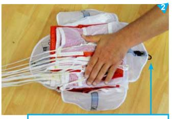
Position the POD's elastic loop opposed to the suspension lines.
