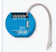
Powerline actuator with 2 channels.  $53x43\,\text{mm}$ ,  $25\,\text{mm}$  deep for mounting in 58 mm switch boxes. Used as impulse switch or relay. 1+1 NO contacts not potential free  $5A/250\,\text{V}$  AC, incandescent lamps 1000 watts. 2 sensor inputs with internal low voltage. Standby loss only 0,5 watt. To control and switch at the same place.
