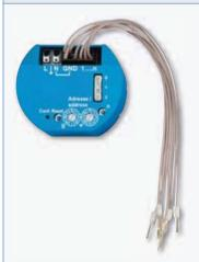
Powerline sensor input with 8 channels. 53x43mm, 25mm deep for mounting in 58mm switch boxes. 8 sensor inputs with internal low voltage. Standby loss only 0,5 watt. To control and switch at different places.
