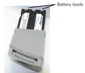
4. Replace the tray, making sure the tray snaps into place. Repeat this process for the other battery tray.
