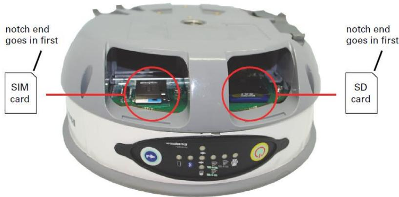
**Note:** When you insert either the SIM card or an SD memory card make sure the contacts on the card are facing the top of the unit and the side of the card with the notch goes in first (see figure above).
