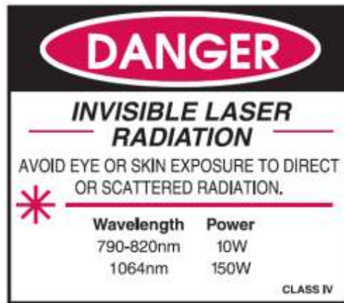
Figure 2-1 Standard Safety Warning Sign
