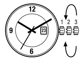
Analog display: Cal. 2824-2 Hours, minutes, seconds. Semi-instantaneous date, date corrector. Winding stem with positions: **Pos. 1** Running position and manual winding. **Pos. 2** Quick correction of date and day. **Pos. 3** Time setting, optional stop-second. Optional stop-second and fine timing devices.
