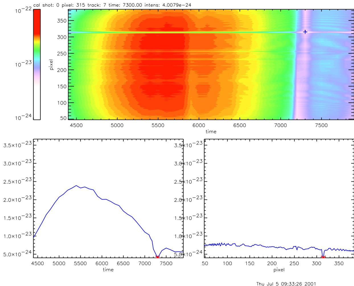
**Fig 3.9: Sensitivity of track7/KS5a displayed with the showspec software (time = wavelength[Å]). “dead” pixel and etaloning can be clearly seen. The lower two graphs show horizontal and vertical sections through the upper graph, taken at the location of the cross.**
