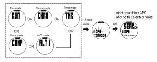
**4.3.3)** Press and hold S7 for 2 seconds from any mode while GPS is initially **OFF**.
