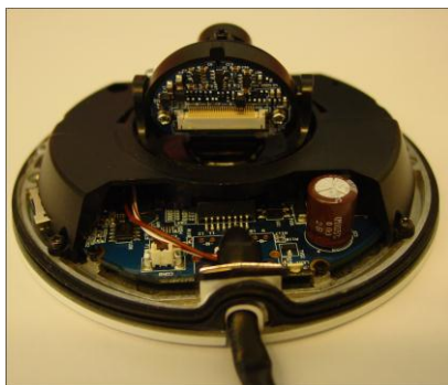
The CD820's waterproof RJ-45 connection
